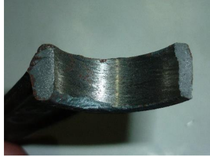
Figure 5. Break point during tensile test.
