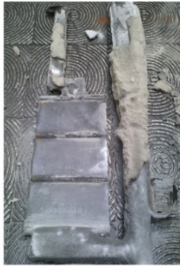
Figure 6. Casting Product for Repaired Modified Design
