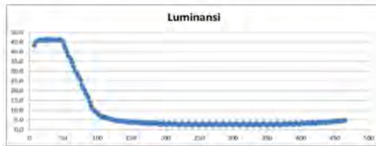
Fig. 10 Simulated luminance level using single-mounted LED lamps
