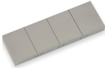
(a) 3-Notch Surface Defect Calibration Standard
