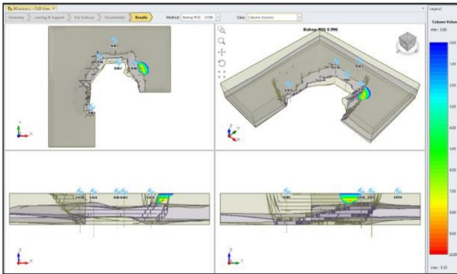
Figure 5. The display of 3D analysis result using Max Columns in X or Y 90 and maximum CS iteration 160
