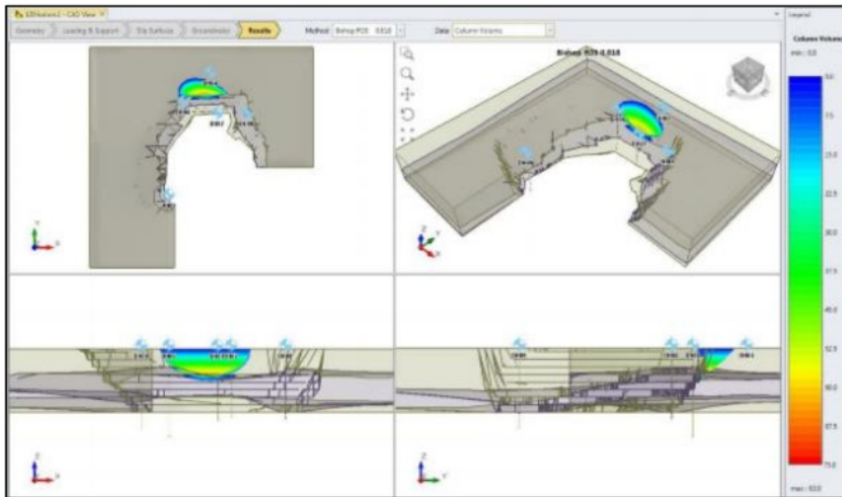
Figure 4. The display of 3D analysis result using Max Columns in X or Y 120 and maximum CS iteration 1200
